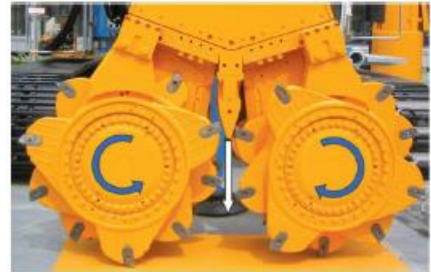
Cutter Soil Mixing (CSM)
